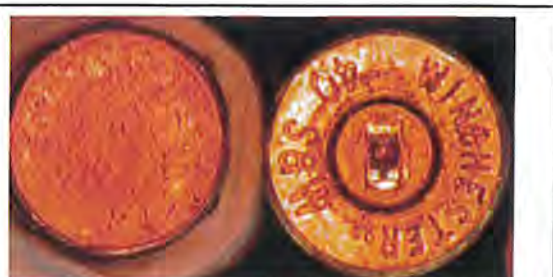
Deputy Kirkpatrick's ammunition- bullet base and cartridge case head stamp and firing pin impression. Note the flat, jacketed base and the rectangular firing pin impression on the cartridge case primer.
