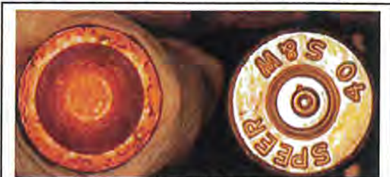
Agent Medlin's ammunition-bullet base and cartridge case head stamp and firing pin impression. Note the concaved, jacketed base of the bullet and the spherical firing pin impression on the cartridge case primer.
