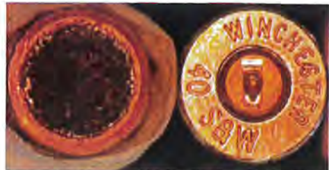
Officer Liles's ammunition- bullet base and cartridge case head stamp and firing pin impression. Note the flat, unjacketed base and the rectangular firing pin impression on the cartridge case primer.
