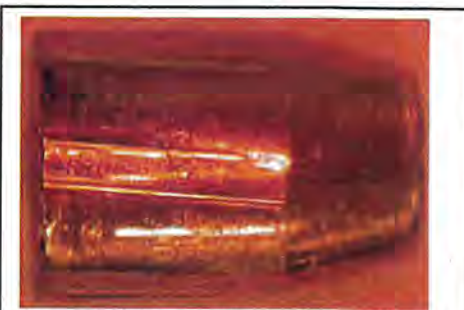
Agent Medlin's ammunition-bearing surface of bullet. Note the well-defined land impressions indicative of conventional barrel rifling.
