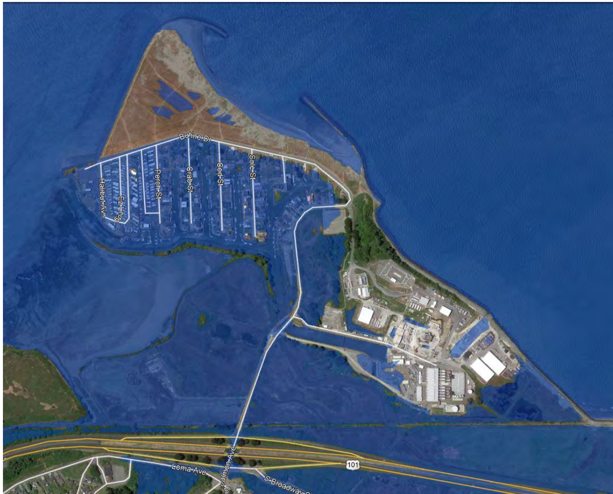
Figure 6. King Salmon potential tidal inundation areas with 1.6 feet (0.5 meter) of sea level rise during a king tide (MAMW) of 10.4 feet, assuming shoreline barrier structures do not exist or are breached. King Salmon Avenue becomes compromised.
