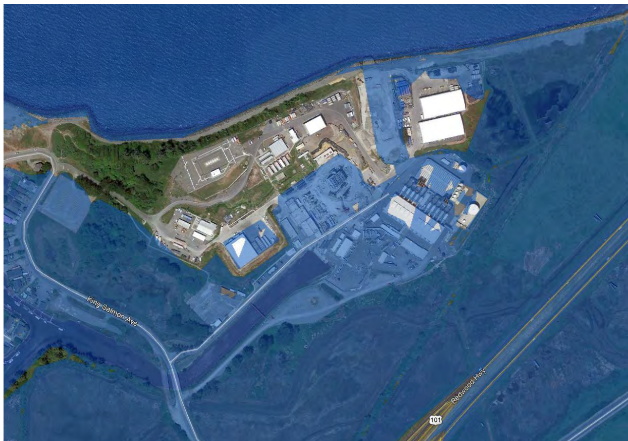
Figure 19. Pacific Gas and Electric Company Humboldt Bay Power Generating Station and facilities in King Salmon with 3.3 feet (1.0 meter) of sea level rise during a king tide, assuming shoreline barrier structures do not exist or are breached.
