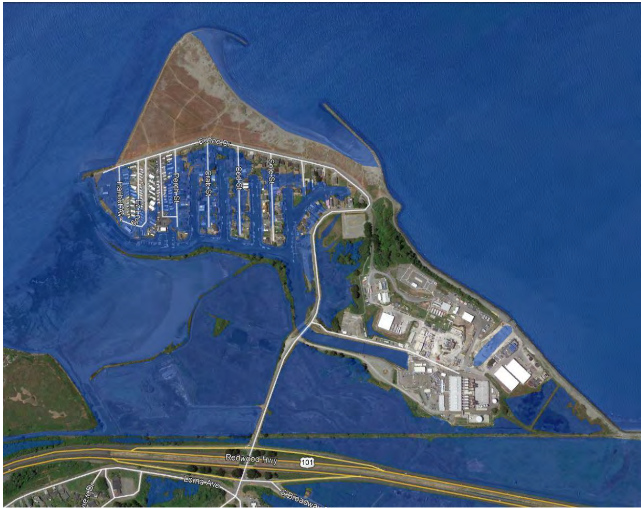
Figure 5. King Salmon potential tidal inundation areas during a king tide (MAMW) of 8.8 feet, assuming shoreline barrier structures do not exist or are breached.
