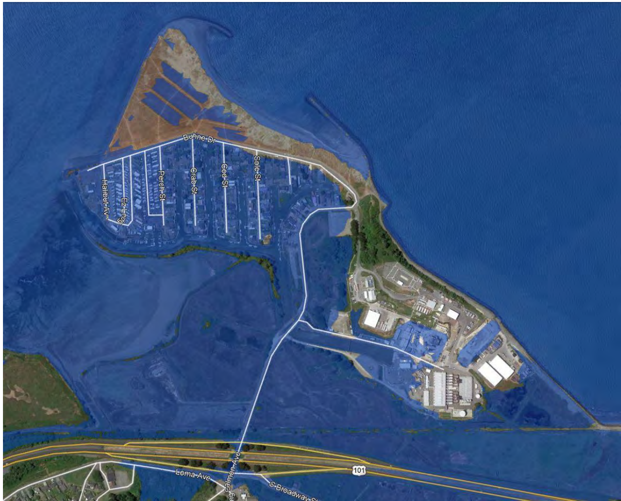
Figure 7. King Salmon potential tidal inundation areas with 3.3 feet (1.0 meter) of sea level rise during a king tide (MMMW) of 11.0 feet, assuming shoreline barrier structures do not exist or are breached. The Humboldt Bay Power Generating Station becomes compromised.
