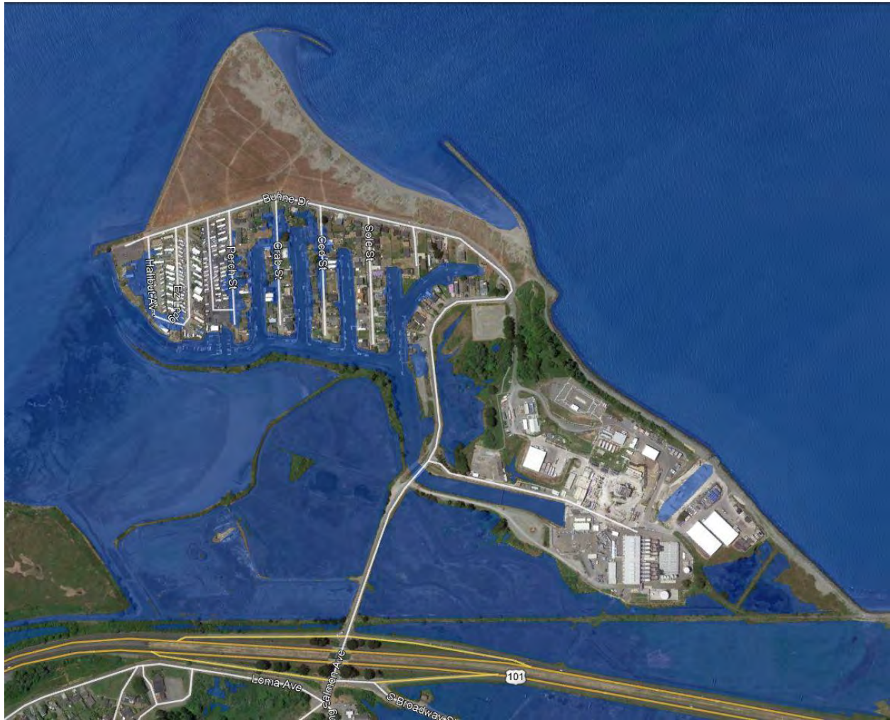
Figure 4. King Salmon potential tidal inundation areas during the daily high tide (MHHW) of 6.5 feet, assuming shoreline barrier structures do not exist or are breached.
