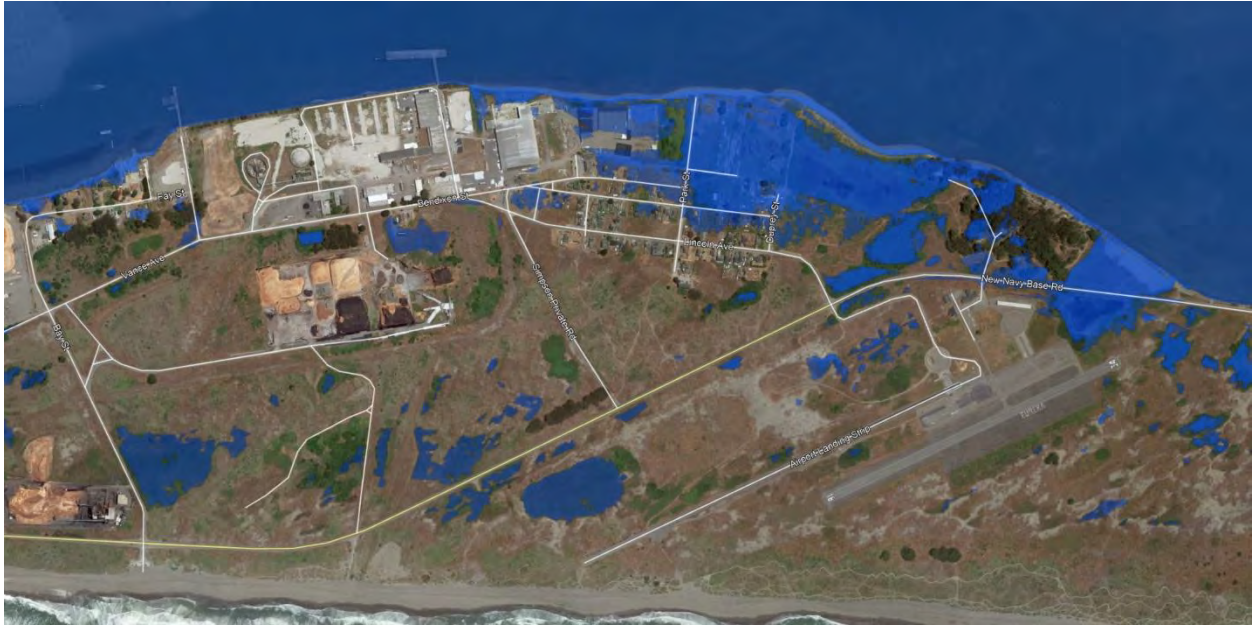
Figure 17. The undeveloped shoreline in Fairhaven and the shoreline in Finntown could be overtopped with 1.6 feet (0.5 meter) of sea level rise (10.4 feet), assuming shoreline barrier structures do not exist or are breached. Residential areas east of Lincoln Avenue could also become tidally inundated 4 to 12 times a year by king tides and monthly maximum tides.
