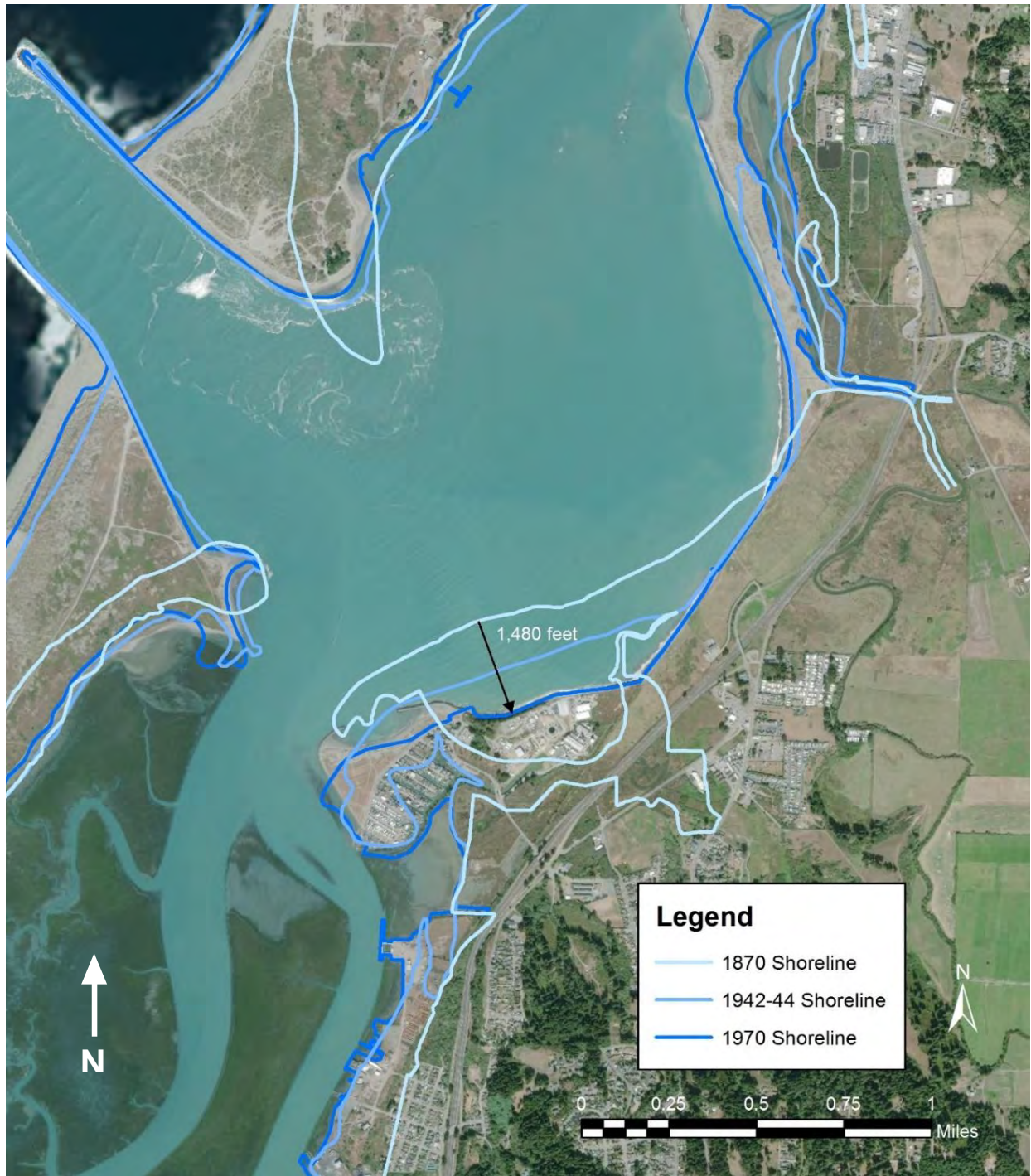
Figure 3. Overlay of erosion of Buhne Hill and shoreline, pre-jetty (1870 shoreline) and post-jetty construction (1940, 1970, and 2017 aerial photographs).
