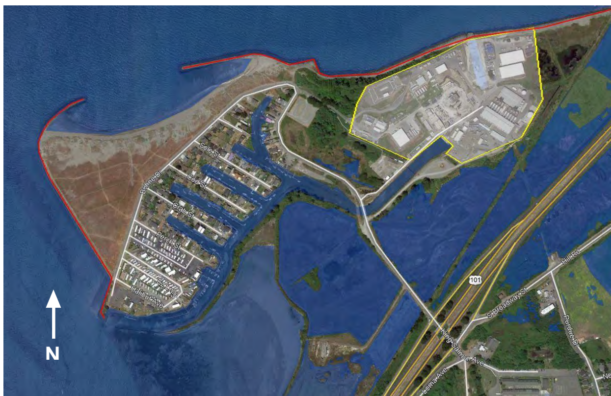
Figure 2. The community of King Salmon, King Salmon Avenue, PG&E facilities (white shading), rock slope protection/jetties (red), and areas inundated by mean higher high water (6.5 feet NAVD 88 measured at the North Spit Tide Gauge).
