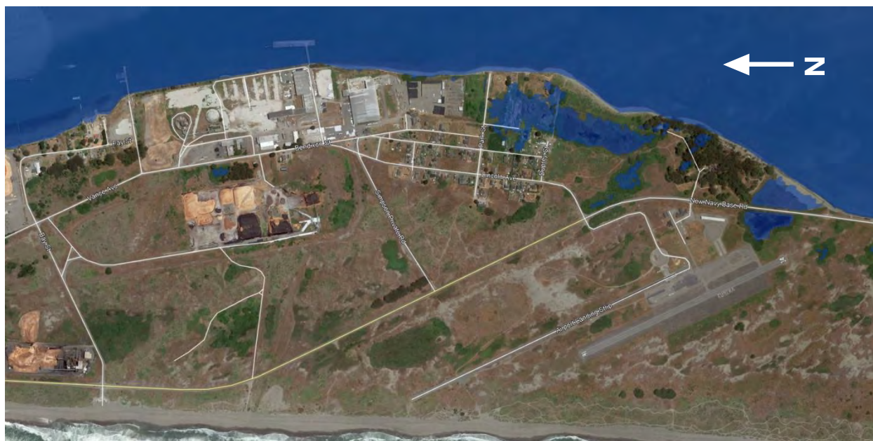
Figure 33. Low-lying areas in and adjacent to Fairhaven (6.5 feet NVAD 88) that are not connected by surface water to the bay.
