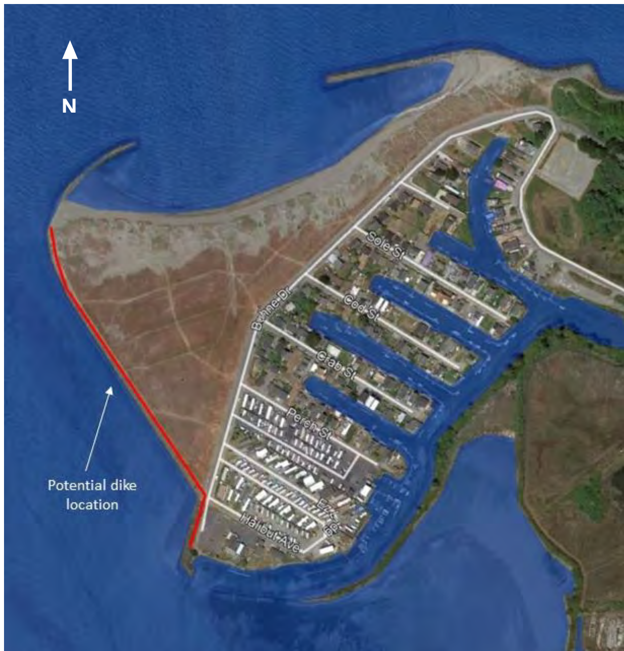
Figure 10. Potential location of a rocky shoreline dike structure approximately 1,600 feet in length to better protect community of King Salmon from tidal inundation.
