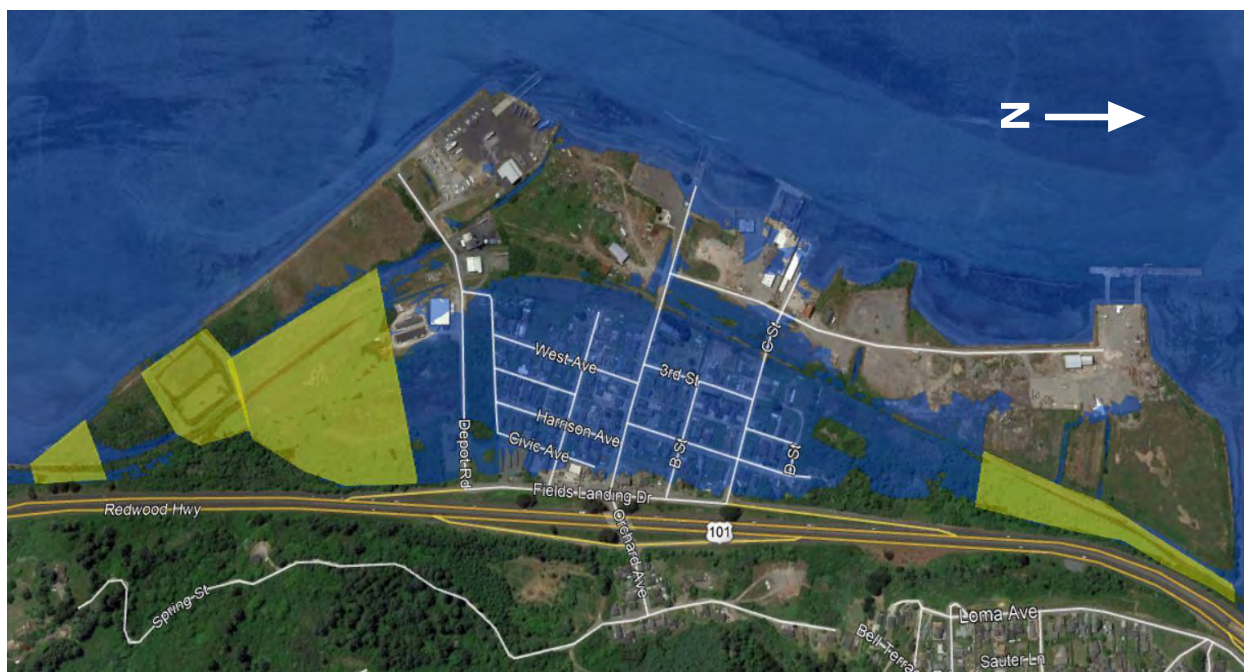
Figure 23. Potential fill barriers (approximately 5 acres in the north and 32 acres in the south) to tidal inundation pathways by MMMW with 1.6 feet (0.5 meter) of sea level rise.
