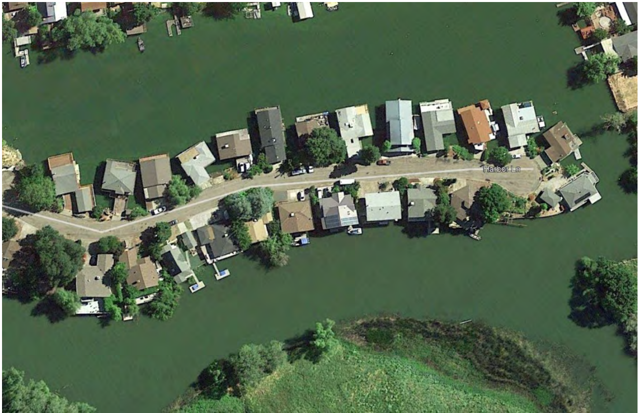
Figure 12. A residential community built on pilings over water, which could be applied in King Salmon to accommodate sea level rise in conjunction with elevated streets.
