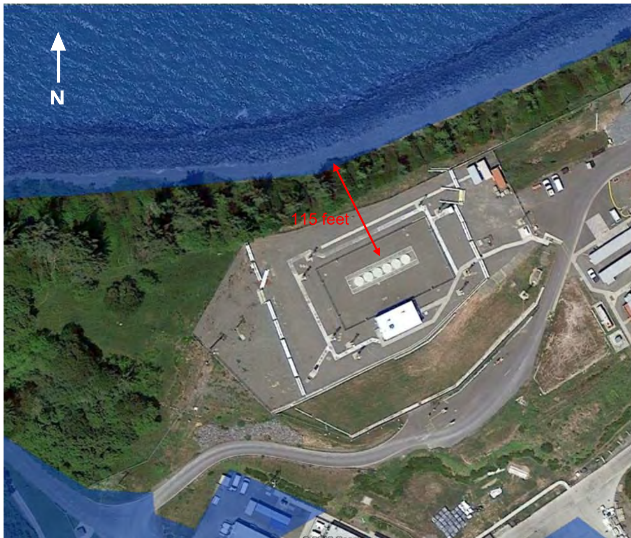
Figure 4. Approximate distance between existing bluff on Buhne Hill and the nuclear Interim Spent Fuel Storage Site is 115 feet. The rock revetment and sea wall would be overtopped by mean annual maximum water or king tides with 6.6 feet (2.0 meters) of sea level rise, assuming the revetment is not raised.
