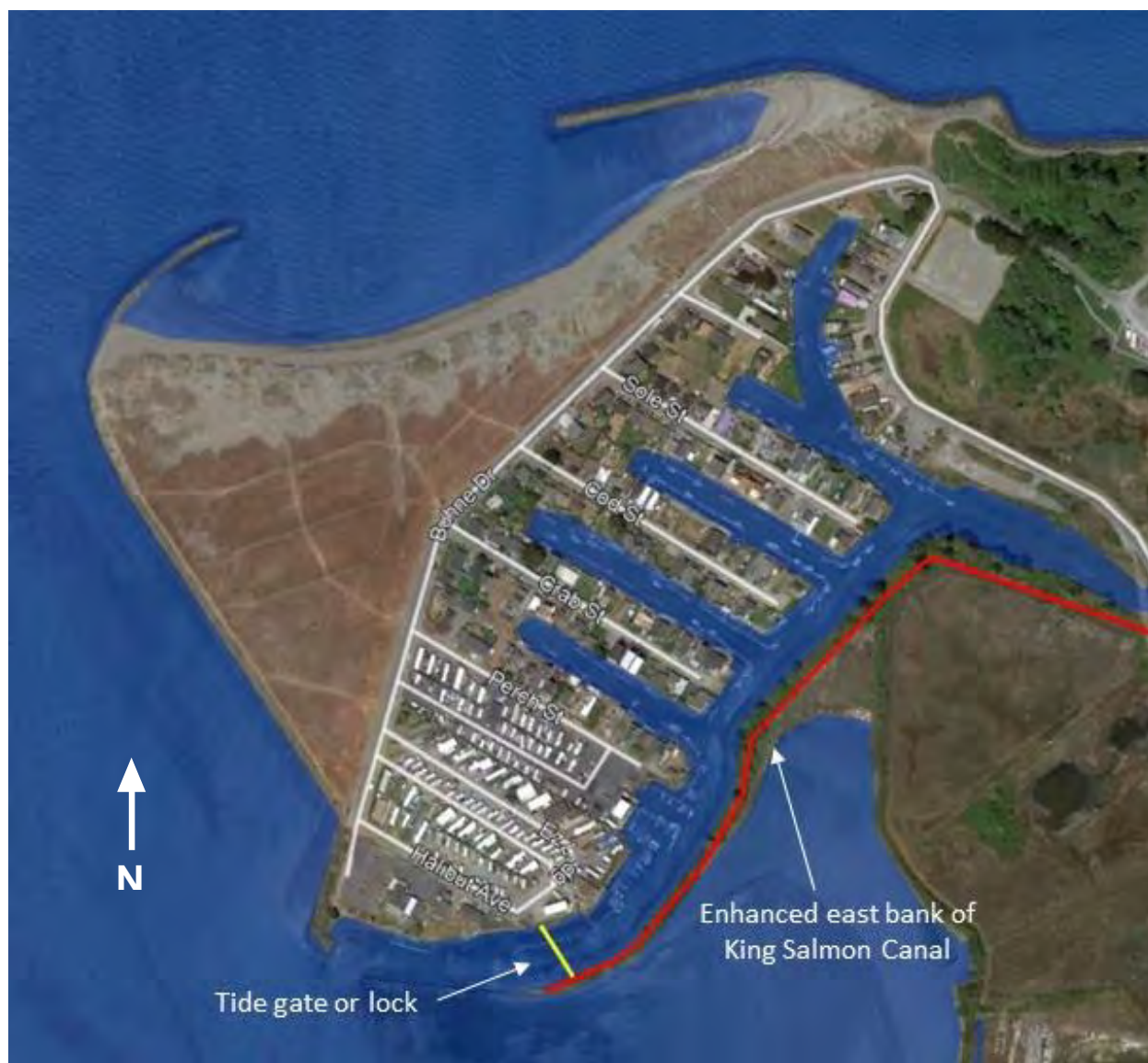
Figure 9. Potential lock-dike structure approximately 2,100 feet in length on the east bank of the King Salmon Canal, and an elevated King Salmon Avenue dike, to protect the community of King Salmon from tidal inundation.
