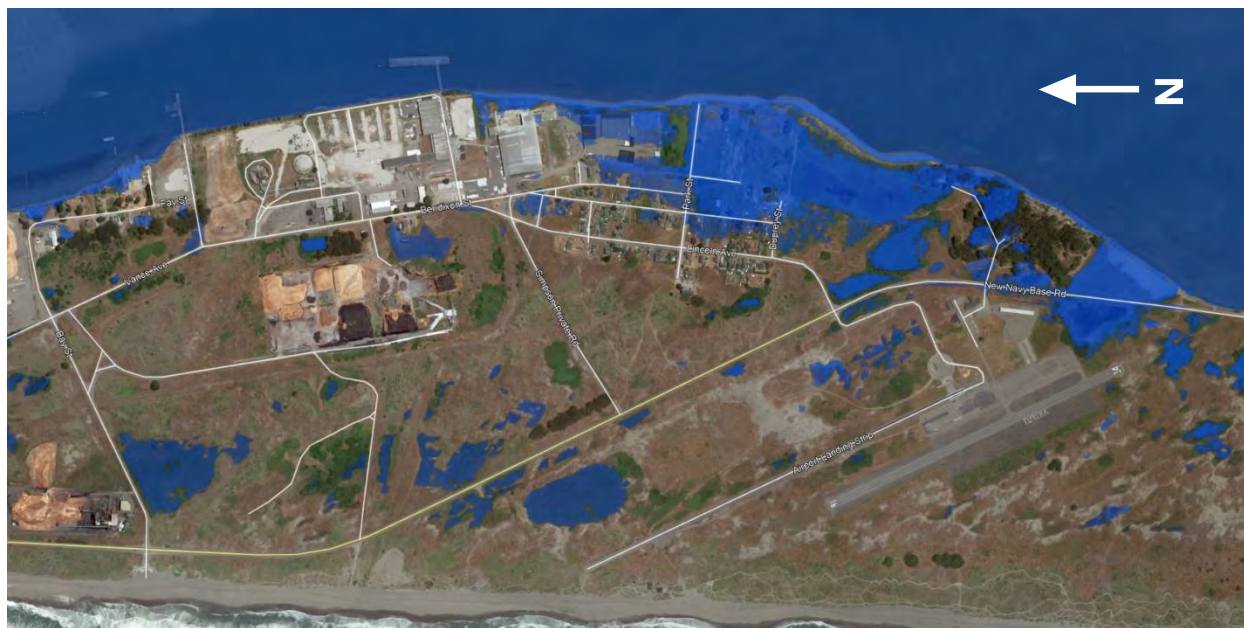
Figure 30. Existing shorelines in Fairhaven and Finntown could be overtopped with 1.6 feet (0.5 meter) of sea level rise combined with a king tide (10.4 feet), assuming shoreline barrier structures do not exist or are breached.
