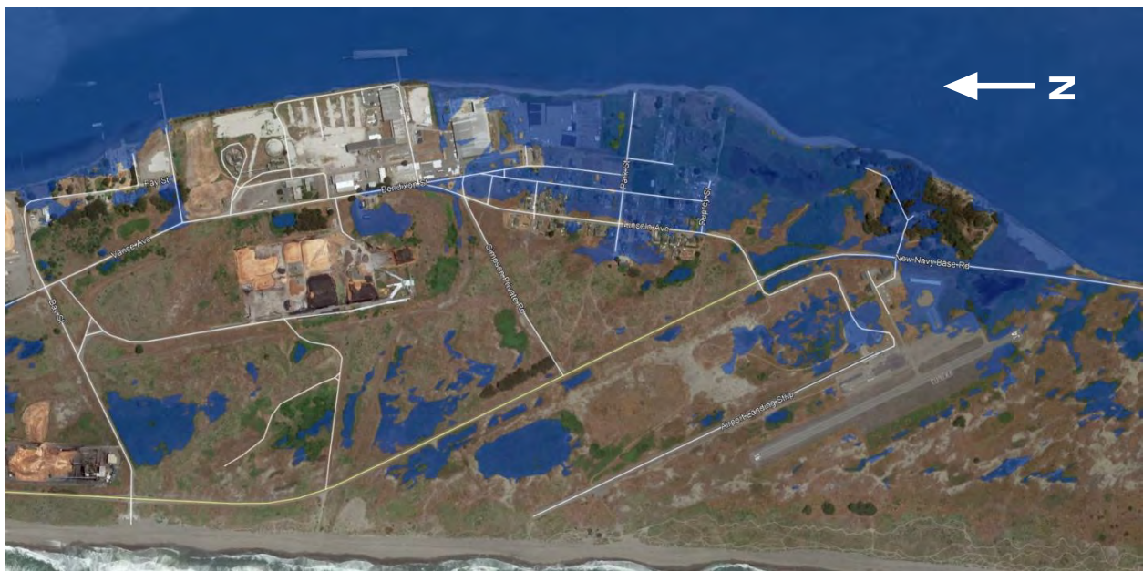
Figure 32. With 4.9 feet (1.5 meter) of sea level rise, MHHW could reach 11.4 feet, nearly all of Fairhaven and Finntown could become tidally inundated daily, assuming shoreline barrier structures do not exist or are breached.
