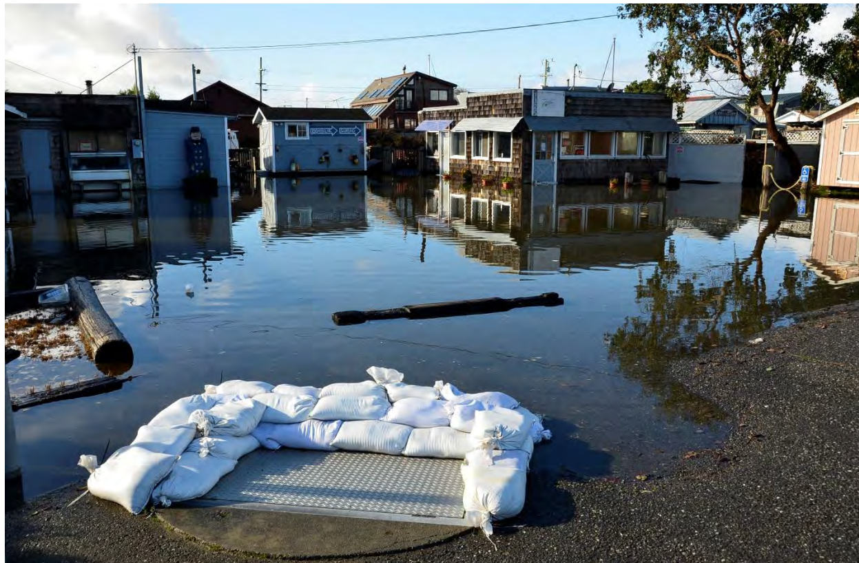
Figure 5. Tidal inundation in King Salmon during a 2017 king tide of 9.4 feet NAVD 88
