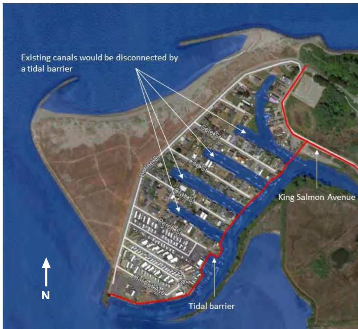
Figure 8. Potential tidal barrier dike structure approximately 2,300 feet in length on the west bank of the King Salmon Canal to protect the community of King Salmon from tidal inundation, and an elevated King Salmon Avenue dike.
