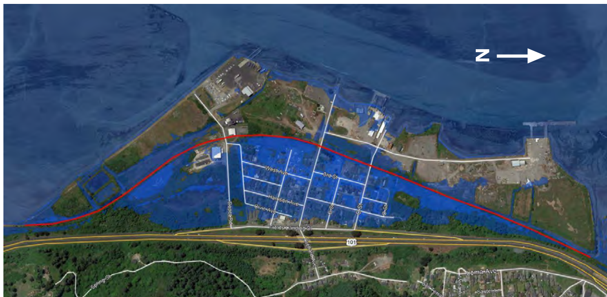
Figure 18. The railroad grade (red line) in Fields Landing provides the primary pathway for tidal inundation of inland, low-lying residential areas by 1.6 feet (0.5 meter) of sea level rise during
