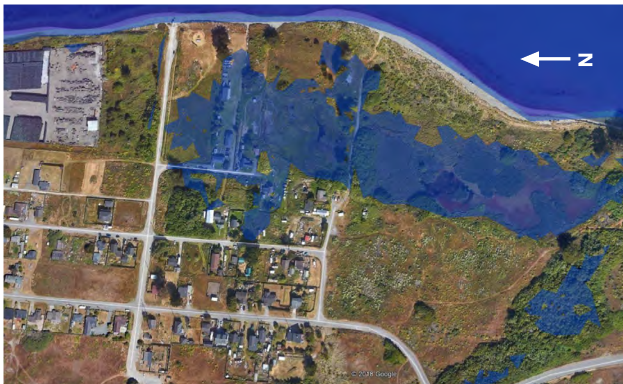
Figure 34. Potential areas in Fairhaven where salt water intrusion could occur when MHHW rises to 8.1 feet, with 1.6 feet (0.5 meter) of sea level rise absent shoreline overtopping.
