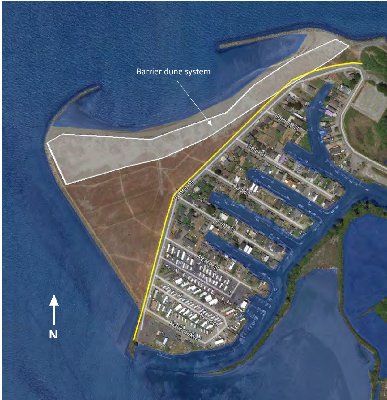
Figure 11. Location of the barrier dune system (approximately 7.8 acres) that protects the community of King Salmon from tidal inundation, and an alternative dike or sea wall protection.
