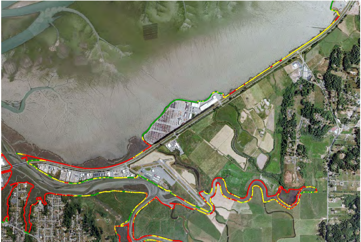
Figure 23. North segment, shoreline vulnerability rating of the lower reach of Highway 101 on Arcata Bay: high (red), moderate (yellow), and low (green) (Laird and Powell 2013).
