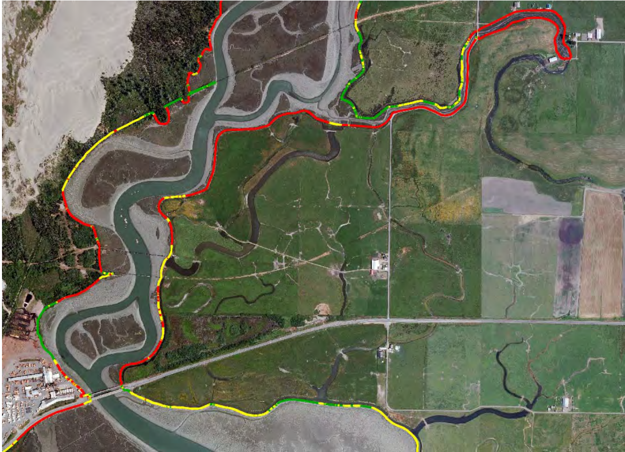
Figure 37. State Highway 255 near Mad River and Liscom Sloughs and dike shoreline vulnerability rating (red=high, yellow=moderate, and green=low).
