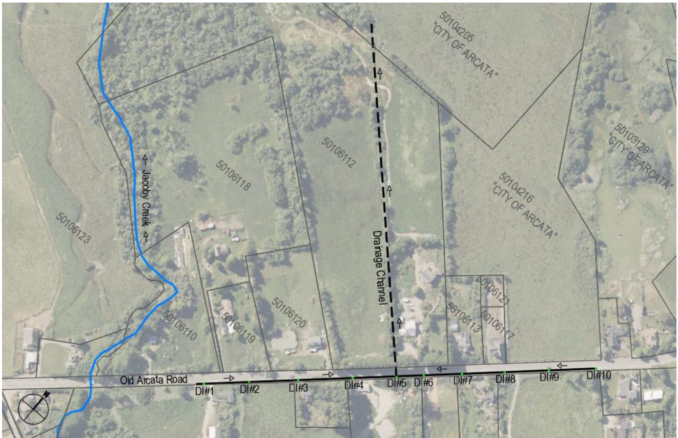
Figure 2 Plan view of existing OAR stormwater system.
