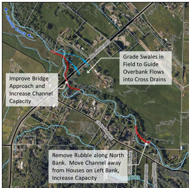
Figure 9-4. Upstream of Baylands 2 -Channel realignment at bridge and upstream meander.
