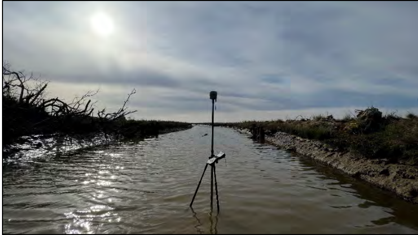
Figure 2-2. RTK rover in Jacoby Creek tidal channel west of US 101
