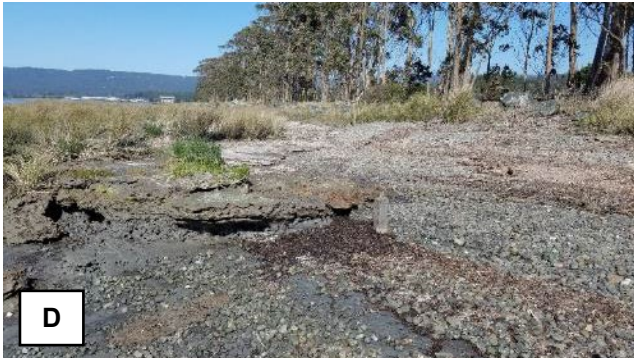
Oblique Photo 4: (A) Deposited railroad ballast gravel in former borrow ditch between rail prisms. (B) Gully/rill bifurcating marsh plain formed parallel to shoreline from frequent runoff of incident wind-wave overtopping and alongshore current. (C) Wood piles understood to have been placed during former oyster farming. (D) thin approximate 2" gravel layer (shingle) overlaid fine sands and silts with transition to marsh scarp and rills formed from marsh plain runoff during wave overtopping events.
