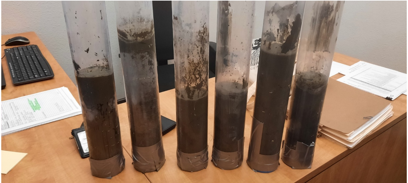
Photo 4. Sample liners with bay mud samples
